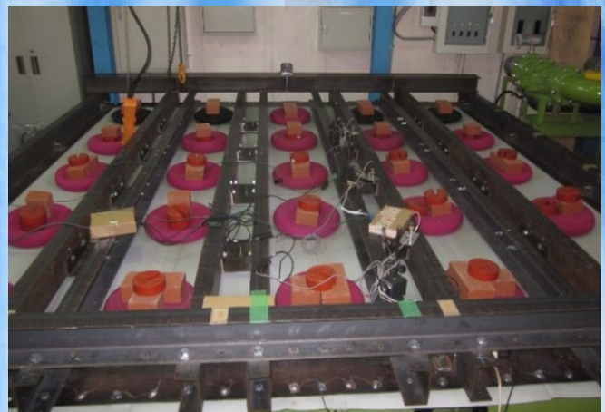
Test of artificial waterproof system with mechanical fixing
