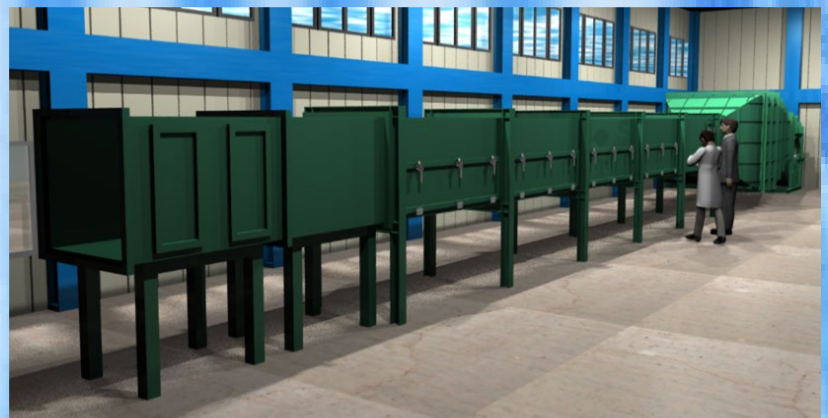
Medium-size turbulent boundary layer wind tunnel
