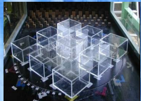
Wind tunnel experiment of natural ventilation
