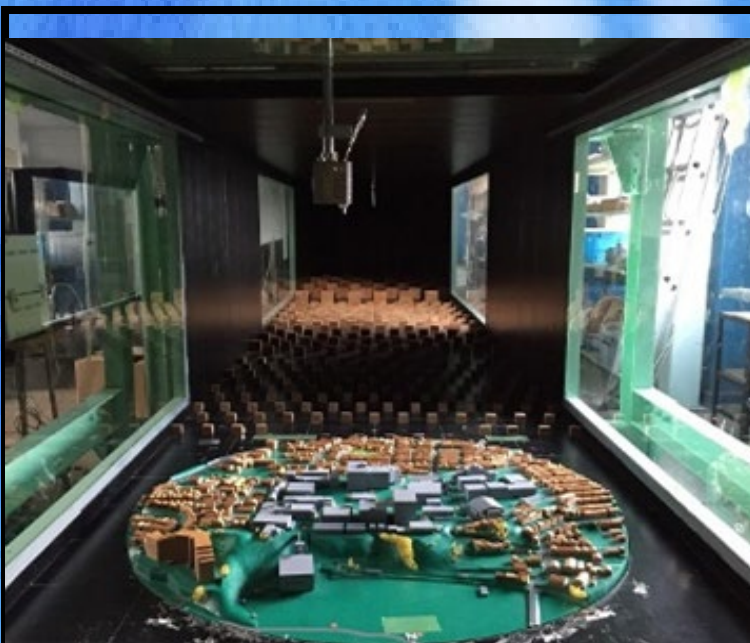
Wind tunnel experiment of pollutant dispersion
