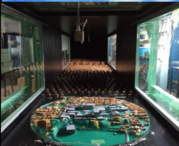
Wind tunnel experiment of pollutant dispersion
