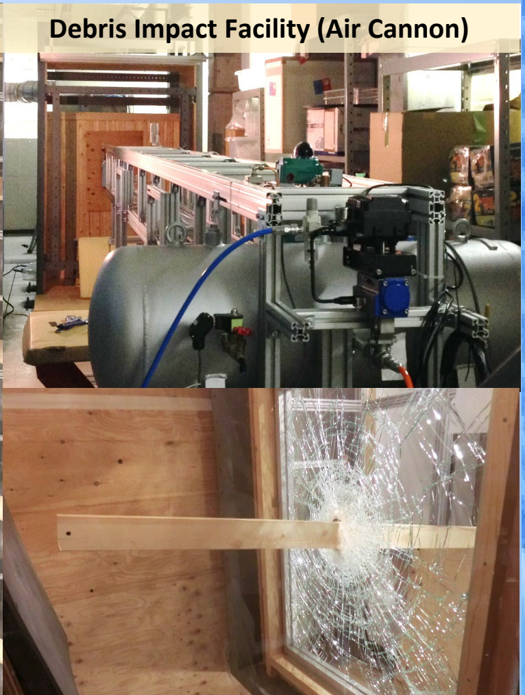
Examples of impact tests on window panes with two-by-four cut pieces of wood Laminated glass reinforced by resin showed impact resistance to flying objects. (pictures on left)
