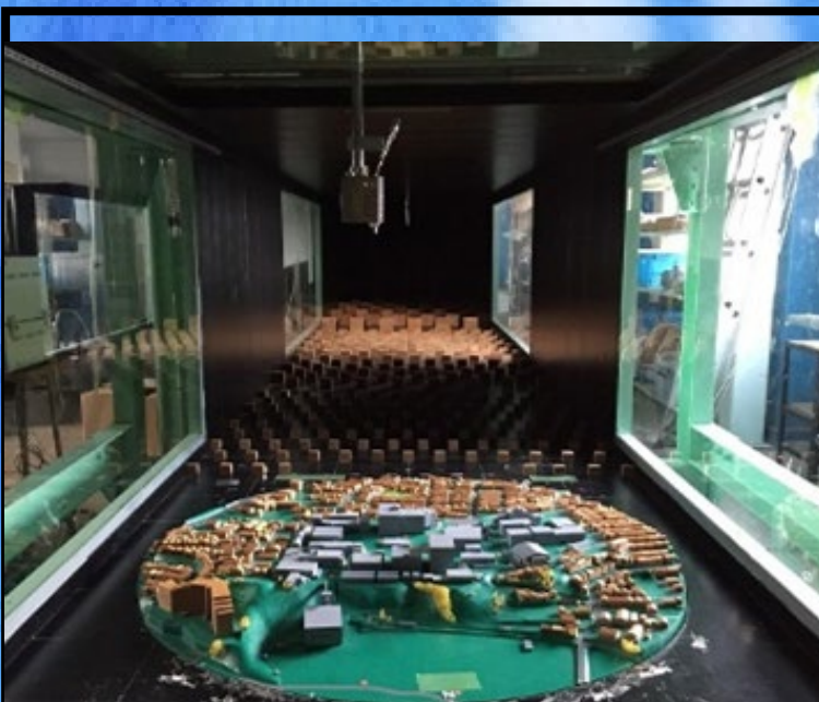
Wind tunnel experiment of pollutant dispersion
