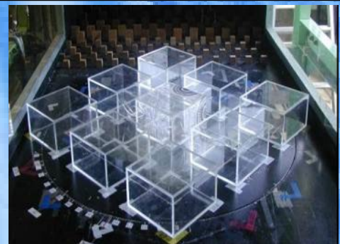
Wind tunnel experiment of natural ventilation
